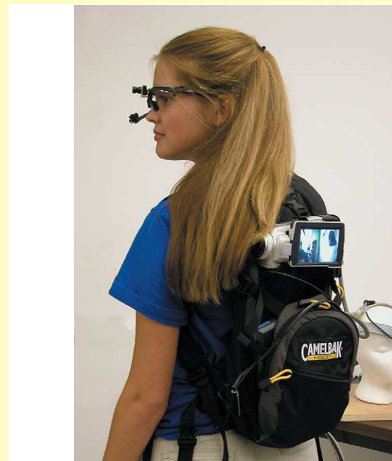
Figure 1. Portable, head mounted eye-tracker developed by Pelz and colleagues [15], based on commercially available systems that use an infrared video camera to image pupil and the corneal reflection. A camera mounted on the frame of the glasses records the scene from the observer's viewpoint. Eye position is then superimposed on the video record.
